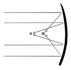
The corrector lens in the MODS camera, and the Schmidt plate in Schmidt—Cassegrain telescopes, compensate for this aberration. The final component is the CCD detector that sits at the focus of the camera, which is located off axis to ensure that the detector does not create a shadow on the mirror.
