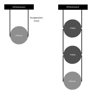
If pendulums are stacked, their attenuation is additive. So by stacking three pendulums with a damping factor of  $10^4$ , we can achieve an attenuation of  $10^{(4+4+4)} = 10^{12}$ . Now we're getting somewhere.
