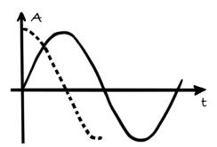
Changes in the length of an arm of the interferometer will lead to a phase shift in the beam that travels along the arm. Because the arms change their length differently, and because the beams started out with zero phase difference because they were "split" from a single laser beam, the relative phasing of the two beams will change, and the resulting interference intensity will
