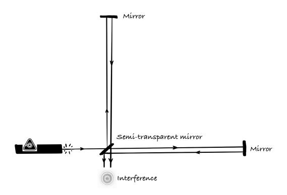
To measure this change in length precisely, you start with a single laser beam, which you then split into two beams using a beamsplitter, basically a semi-transparent mirror. You then send the two beams along the two roughly perpendicular arms: these are 600 meters long for GEO600 and 4,000 meters for LIGO. A mirror at the end of each arm reflects the light back. Because of
